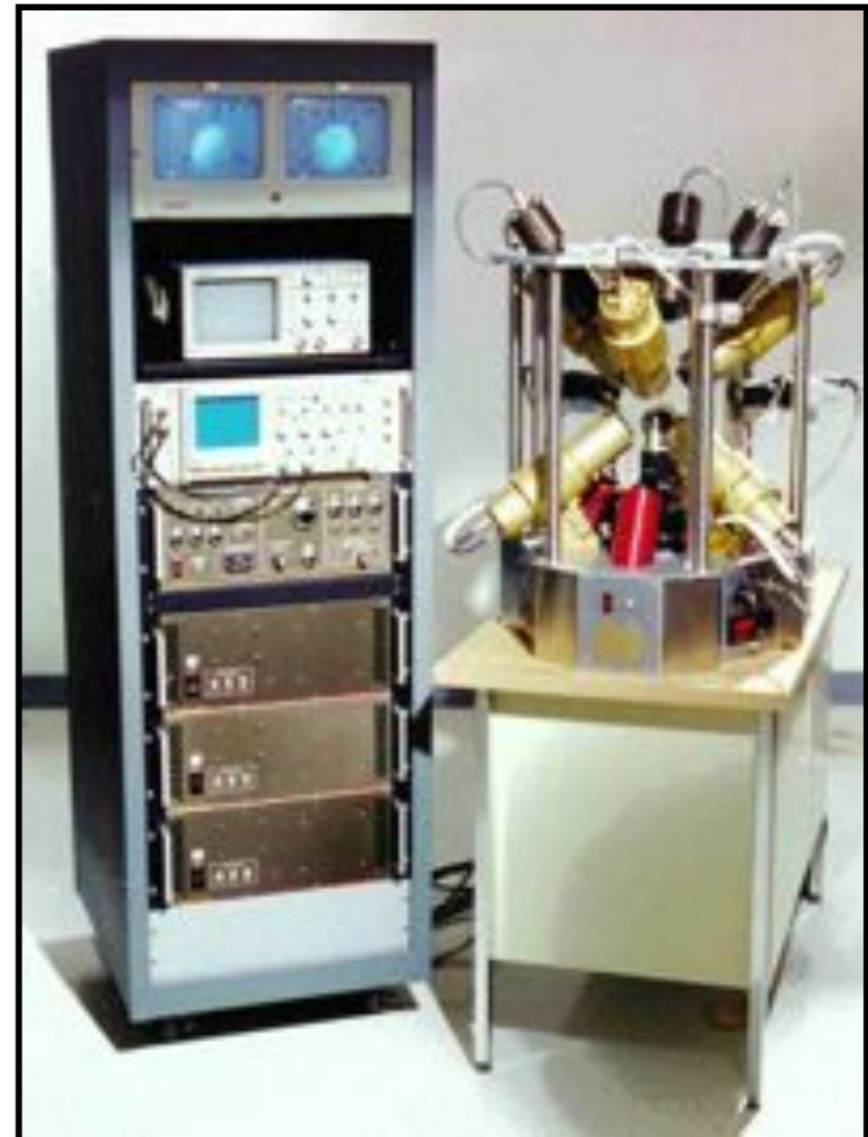
Photograph of the Aero-Acoustic Levitator showing table-top mounted levitation system and instrument rack holding acoustic power supplies, levitator controller electronics, and video monitors.
